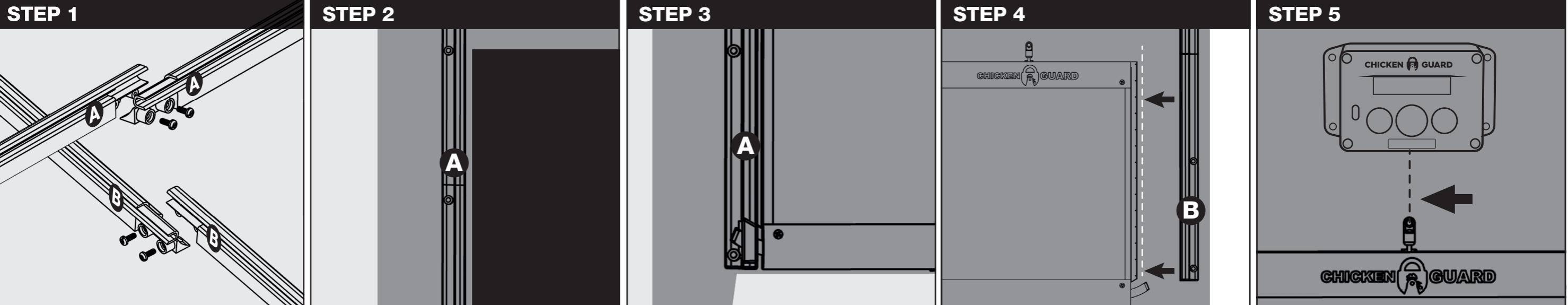
Align both 'A' runners & secure with 2 'small' screws. (repeat procedure for 'B' runners)
